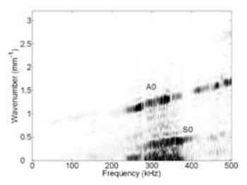
Fig. 5- Reinforcement of the symmetric Lamb mode and cancellation of the antisymmetric one by exciting the two actuators in phase.
