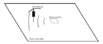
Fig. 1- Ceramic position on the aluminum plate.
