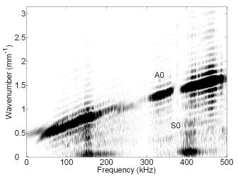
Fig. 6- Reinforcement of the antisymmetric Lamb mode and cancellation of the symmetric one by exciting the two actuators out of phase.
