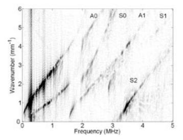
Fig. 3- Experimental dispersion curves for an aluminum plate of thickness 2h calculated applying the 2D FFT algorithm to the data measured with the needle hydrophone.
