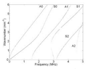
Fig. 2- Analytical dispersion curves for an aluminum plate of thickness 2h obtained solving the Rayleigh-Lamb equations.
